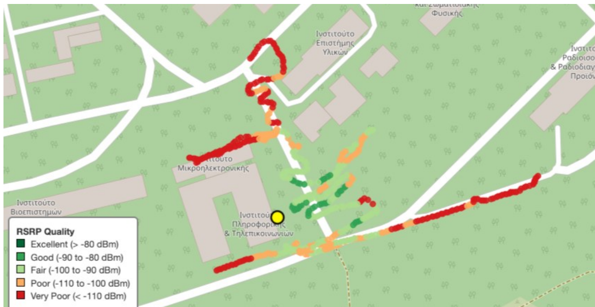
Figure 16: Spatial distribution of predicted RSRP values across the deployment area. The yellow dot indicates the antenna location
