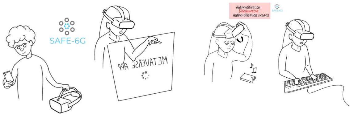
Figure 4: Users both connect their XR headsets to the SAFE-6G network and then authenticate themselves on the metaverse application. Removing the headset at any time locks the metaverse application. The user will need to be re-authenticated each time.
